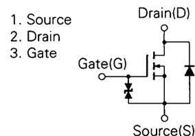
(Diode in the figure is the parasitic diode.)
