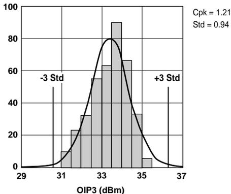
**Figure 3. OIP3 @ 2 GHz, 4 V, 80 mA.**
