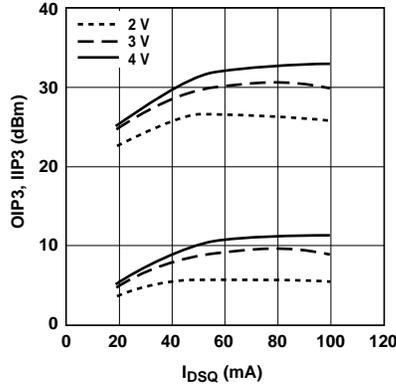
Figure 7. OIP3, IIP3 vs. Bias<sup>[1]</sup> at 900 MHz.
