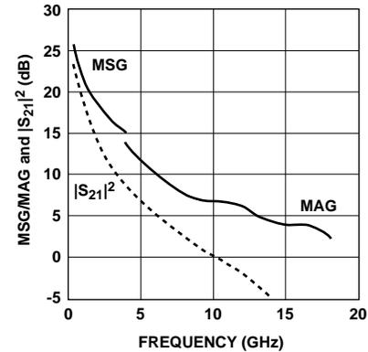
Figure 21. MSG/MAG and  $|S_{21}|^2$  vs. Frequency at 4V, 60 mA.
