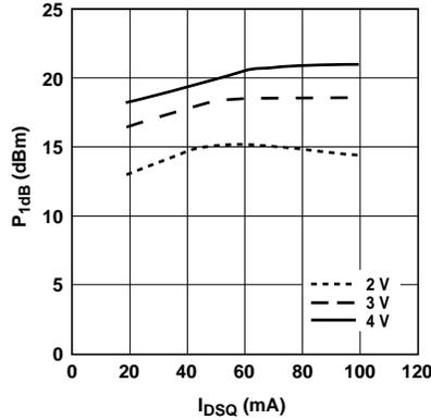
Figure 9. P<sub>1dB</sub> vs. Bias<sup>[1,2]</sup> Tuned for NF @ 4V, 80 mA at 900 MHz.
