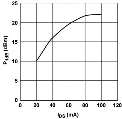
Figure 18. P<sub>1dB</sub> vs. I<sub>DS</sub> Active Bias<sup>[1]</sup>
