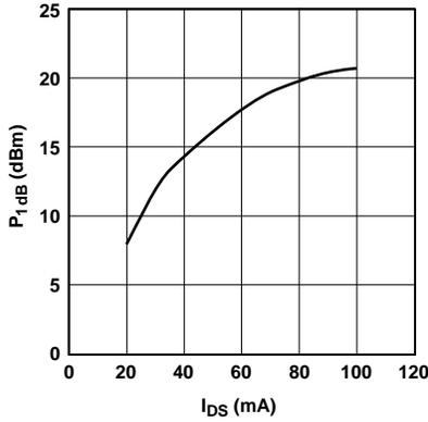
Figure 19. P<sub>1dB</sub> vs. I<sub>DS</sub> Active Bias<sup>[1]</sup>
