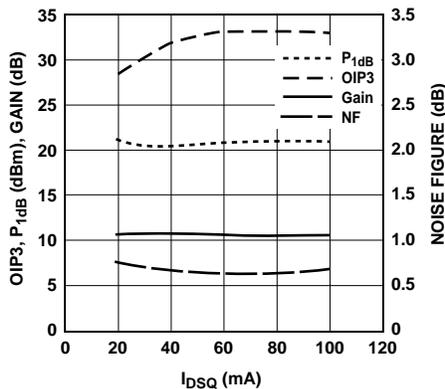
Figure 16. OIP3,  $P_{1dB}$ , NF and Gain vs. Bias<sup>[1,2]</sup> at 3.9 GHz.
