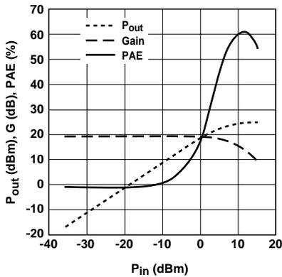
**Figure 20. Swept Power Tuned for Max  $P_{1dB}$**
