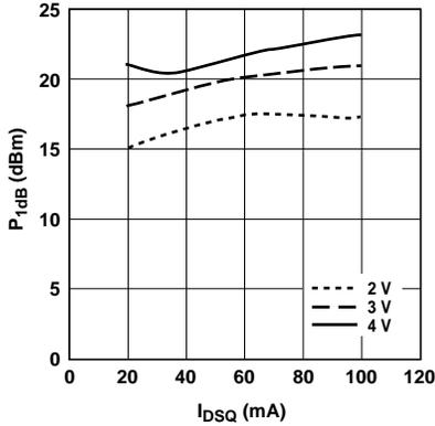
Figure 8. P<sub>1dB</sub> vs. Bias<sup>[1,2]</sup> at 2 GHz.
