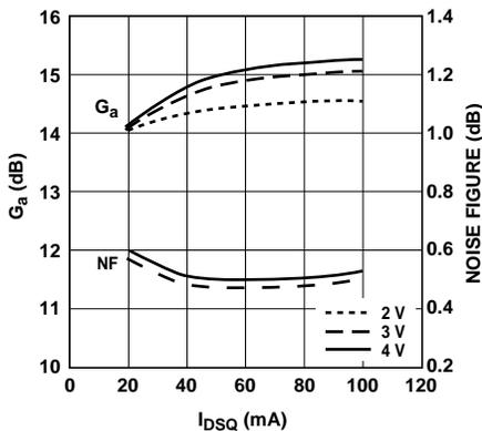
Figure 10. NF and  $G_a$  vs. Bias<sup>[1]</sup> at 2 GHz.
