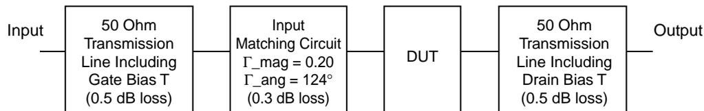
Figure 5. Block diagram of 2 GHz production test board used for Noise Figure, Associated Gain,  $P_{1dB}$ , and OIP3 measurements. This circuit represents a trade-off between an optimal noise match and a realizable match based on production test requirements. Circuit losses have been de-embedded from actual measurements.
