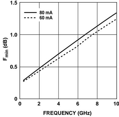
Figure 12.  $F_{min}$  vs. Frequency and Current at 4V.
