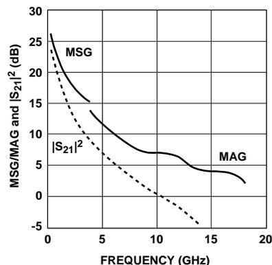
**Figure 22. MSG/MAG and  $|S_{21}|^2$  vs. Frequency at 4V, 80 mA.**
