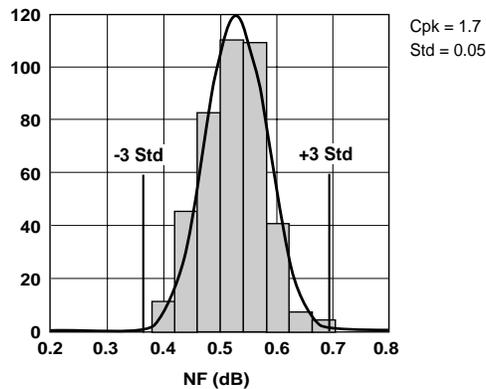
**Figure 2. NF @ 2 GHz, 4 V, 80 mA.**
