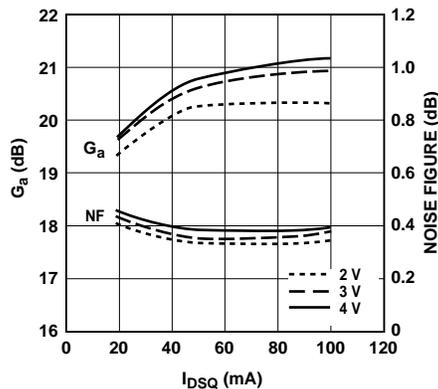
Figure 11. NF and  $G_a$  vs. Bias<sup>[1]</sup> at 900 MHz.
