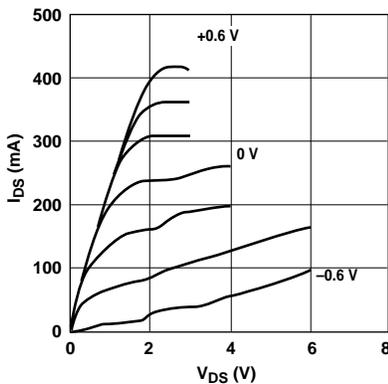
**Figure 1. Typical Pulsed I-V Curves<sup>[7]</sup>.**
