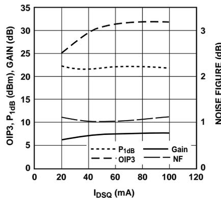
Figure 17. OIP3,  $P_{1dB}$ , NF and Gain vs. Bias<sup>[1,2]</sup> at 5.8 GHz.
