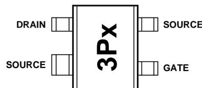
**Note:** Top View. Package marking provides orientation and identification.
