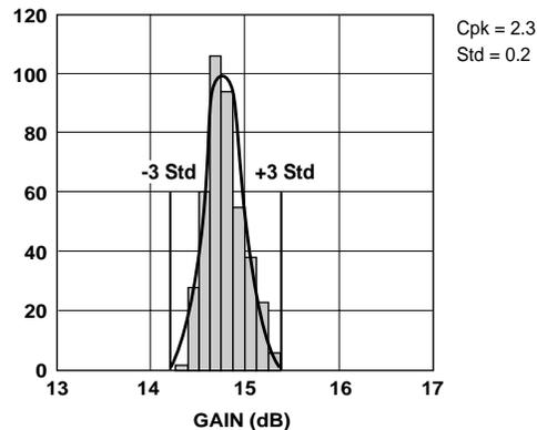
**Figure 4. Gain @ 2 GHz, 4 V, 80 mA.**
