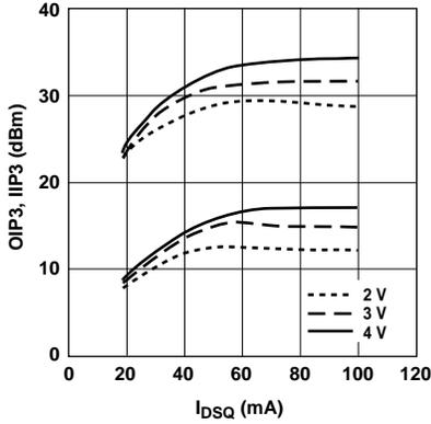
Figure 6. OIP3, IIP3 vs. Bias<sup>[1]</sup> at 2 GHz.
