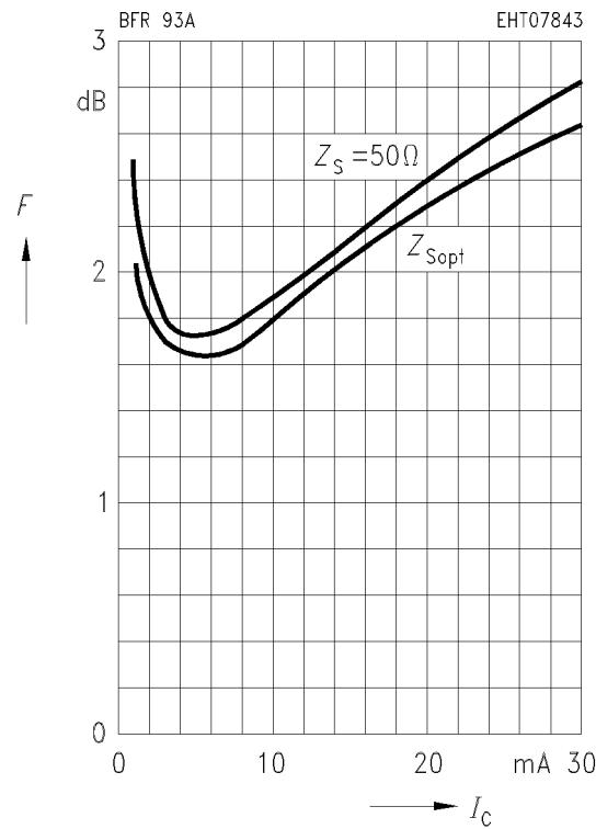
**Noise figure  $F = f(I_C)$**  $V_{CE} = 8 \text{ V}, f = 2 \text{ GHz}, Z_{\text{Lopt}} (G)$
