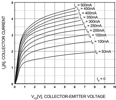
**Figure 1. Static Characteristic**
