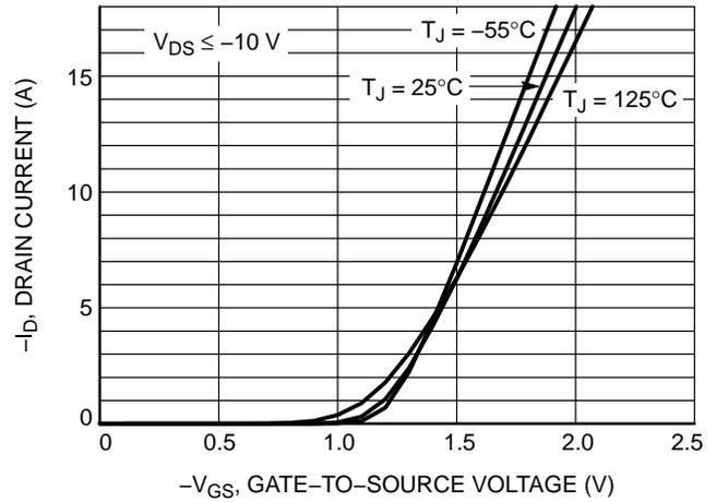
Figure 2. Transfer Characteristics
