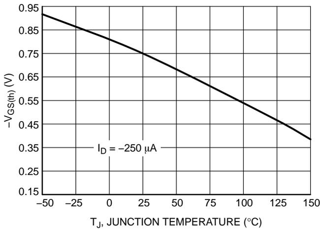
Figure 11. Threshold Voltage
