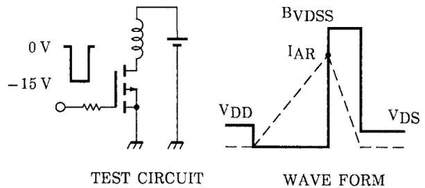
$T_{ch} = 25^\circ\text{C}$  (Initial)
