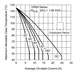
Fig. 2 - Current Ratings Characteristics
