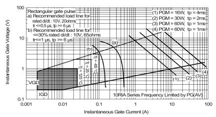
Fig. 9 - Gate Characteristics
