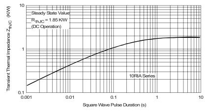
Fig. 8 - Thermal Impedance Z<sub>thJC</sub> Characteristics
