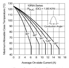
Fig. 1 - Current Ratings Characteristics
