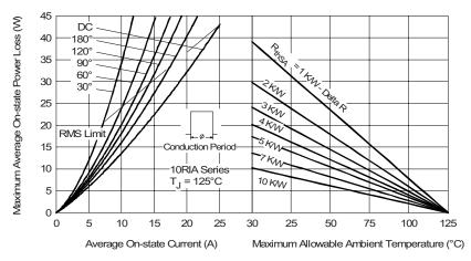
Fig. 4 - On-State Power Loss Characteristics
