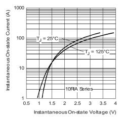
Fig. 7 - Forward Voltage Drop Characteristics
