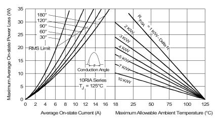
Fig. 3 - On-State Power Loss Characteristics
